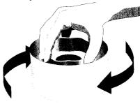
5. Place sealing ring in lid and press firmly in place, being sure to engage ring under tabs.
