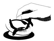
3. Place the blade assembly with the sealing ring in the bottom opening of the jar. Use caution.
